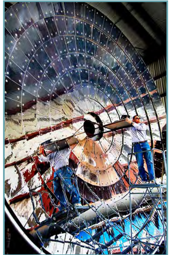
Sandia Labs is testing whether solar power may be used to transform CO 2 into carbon monoxide, which can be converted to methanol, jet fuel, or gasoline.
