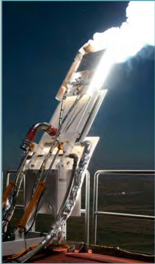
Solar power heats NASA space shield material. The tests at Sandia Labs apply heat equivalent to 1,500 suns to spacecraft shields
