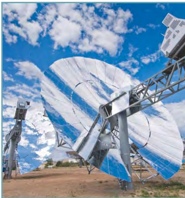
The SunCatcher™, newly designed solar power collection dishes at Sandia's National Solar Thermal Test Facility. Designed for high-volume production, ease of maintenance, and cost reductions, the dishes could be in commercial service by 2010.
